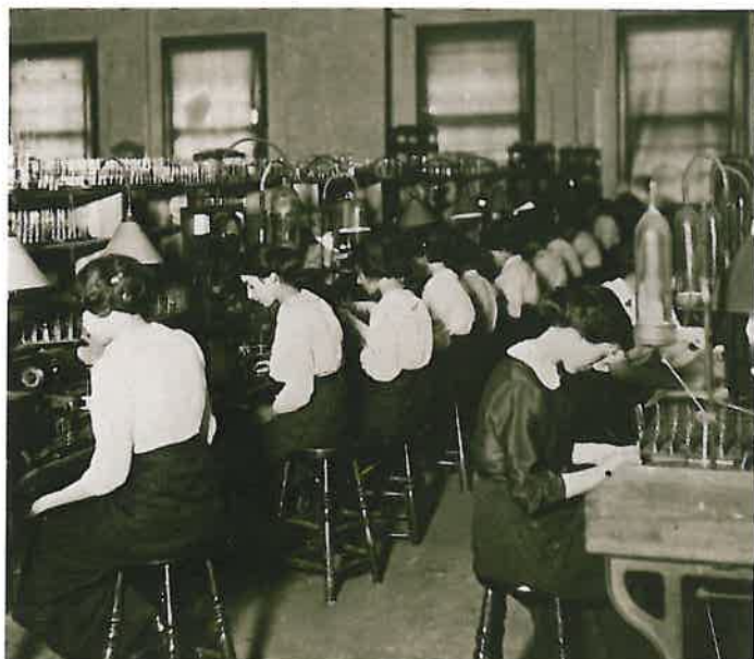
In 1910, tungsten filament lamps were still assembled by hand and the bulbs blown individually, shown below; a typical industrial installation of the time is shown in the upper right-hand picture.
