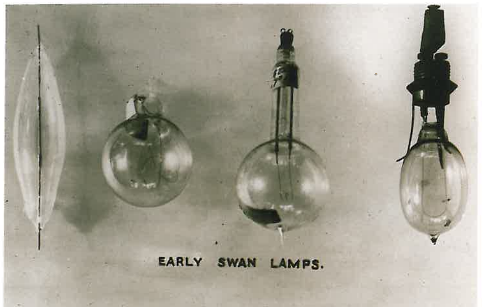
Some early Swan lamps. Swan's original lamp is on the left of the group.
