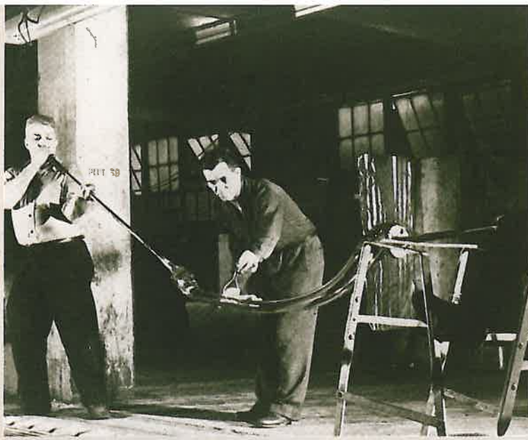
Blowing the glass tubing for fluorescent lamps was still a craft operation in the forties. The lamps themselves were assembled by hand. The picture shows capping and ageing lamps.
